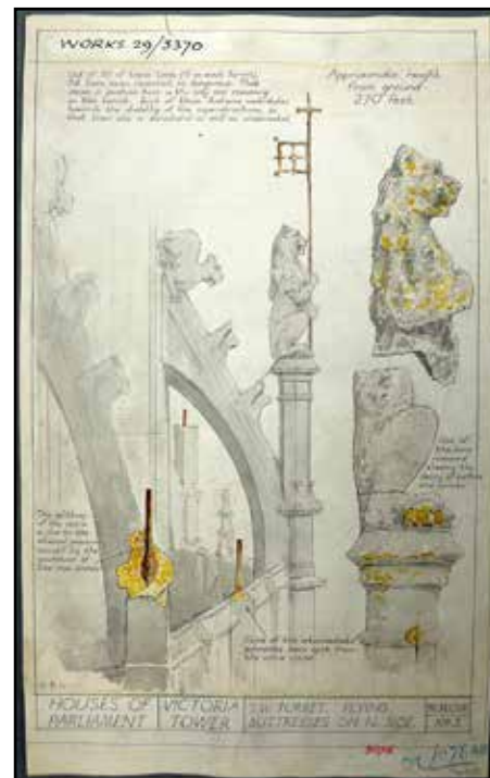
A water-coloured drawing used to illustrate the damage in the 1920s.
